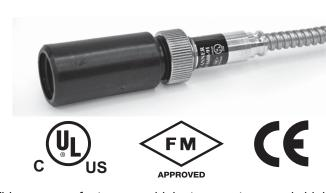
This sensor features a high temperature and high sensitivity ultraviolet (UV) tube for monitoring gas or oil flames which cycle on and off frequently. The Eclipse flame safeguard checks for a short-circuited, or "runaway" scanner at the beginning and end of each flame cycle.
